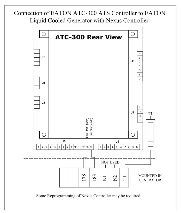
Figure 6. Connection of EATON ATC-300 ATS Controller to Eaton Liquid Cooled Generator with Nexus Controller.
