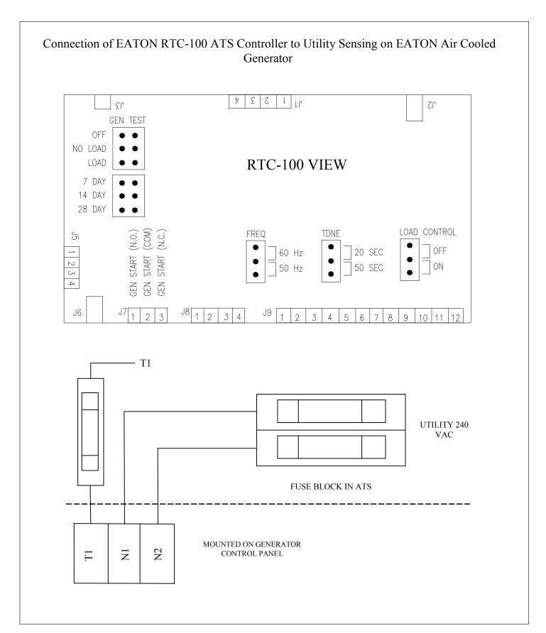
Figure 3. Connection of EATON RTC-100 ATS Controller to Utility Sensing on EATON Air Cooled Generator with Nexus Controller.
