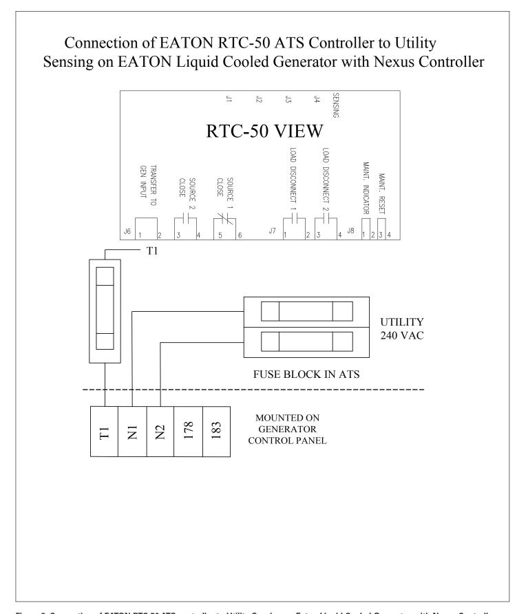
Figure 2. Connection of EATON RTC-50 ATS controller to Utility Sensing on Eaton Liquid Cooled Generator with Nexus Controller.
