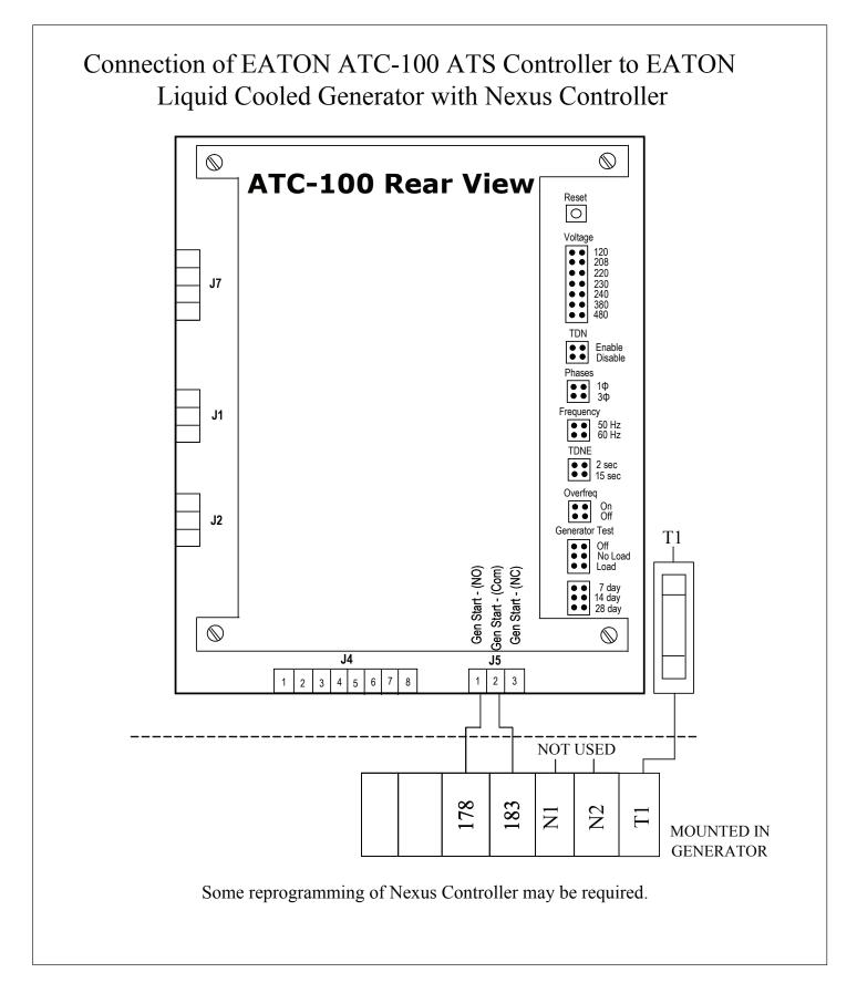
Figure 5. Connection of EATON ATC-100 ATS Controller to Eaton Liquid Cooled Generator Controller with Nexus Controller.
