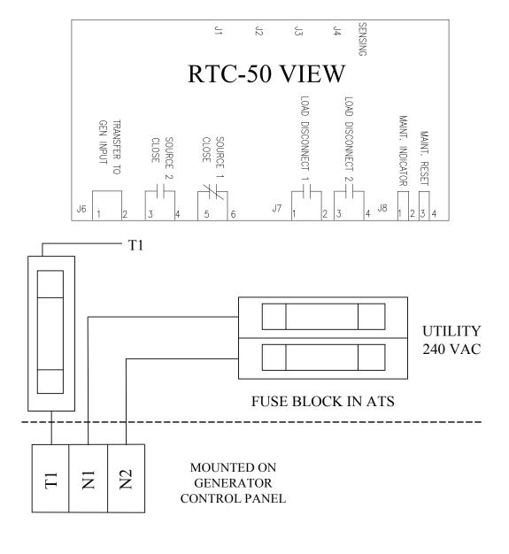
Figure 1. Connection of EATON RTC-50 ATS Controller to Utility Sensing on EATON Air Cooled Generator with Nexus Controler.
