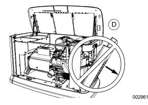
Figure 2-5. Intake Side Panel Removal
