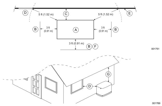
Figure 3-1. Installation Clearances
