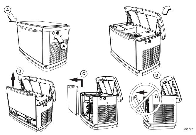
Figure 2-4. Side Lock Location and Front Panel Removal
