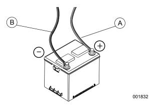
Figure 6-2. Battery Cable Connections
