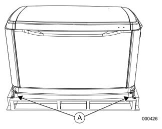
Figure 2-2. Generator on Pallet
