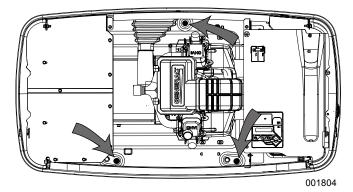
Figure 4-2. Mounting Hole Location
