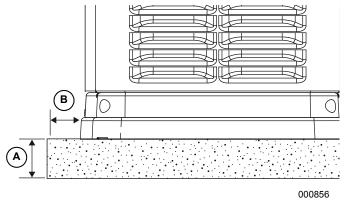
Figure 3-3. Compacted Soil or Gravel Pad
