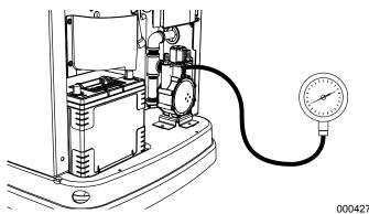
Figure 5-4. Checking Pressure with Manometer
