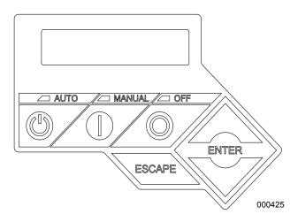
Figure 7-1. Generator Control Panel
