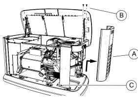
**3.** Lift the intake panel up and away from the generator.
