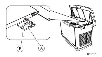
Figure 2-8. Generator Main Line Circuit Breaker
