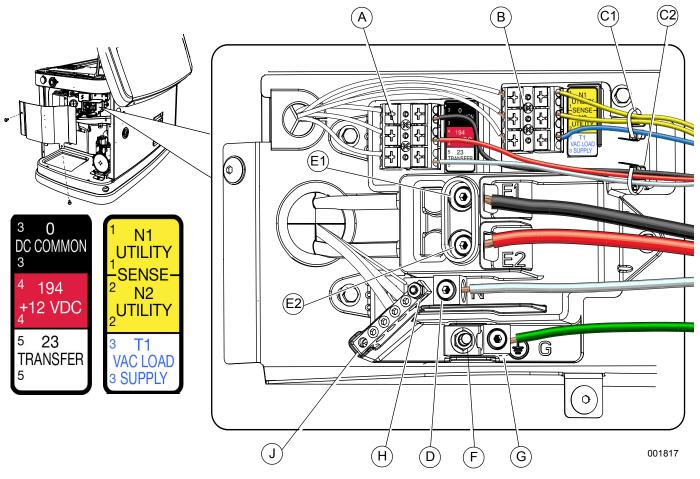
Figure 6-1. I Electrical Wiring Connections
