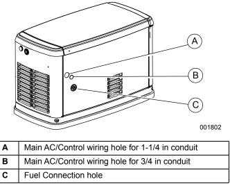
Figure 2-7. Rear Connections
