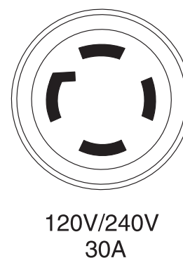
Figure 7 - 120/240 VAC, 30 Amp Receptacle
