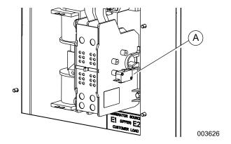
Figure 3-3. Auxiliary Contact
