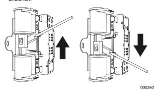
Figure 4-1. Manual Transfer Switch Operation
