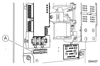
Figure 4-2. Fuse Removal and Installation Tool
