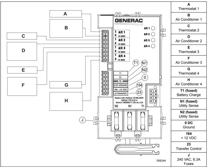
Figure 3-3. Typical SACM Connections
