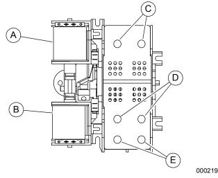
Figure 2-1. Typical Single-Phase ATS Transfer Mechanism
