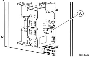
Figure 3-4. Auxiliary Contact
