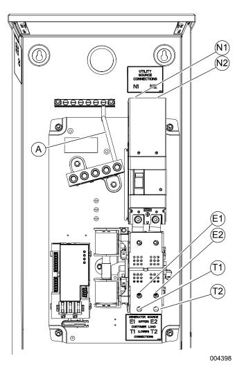
Figure 3-2. Wiring Connections
