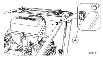
Figure 3-7. Internal Auxiliary Shutdown Switch (13–22kW)
