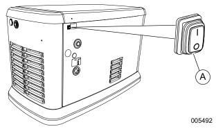
Figure 3-6. External Auxiliary Shutdown Switch (all models)
