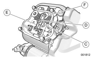
Figure 4-7. Valve Clearance Adjustment (10 kW)
