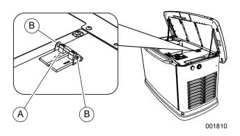
Figure 3-4. Main Line Circuit Breaker (MLCB)
