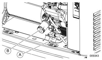
Figure 4-3. Oil Filter and Drain Location (20–22 kW)
