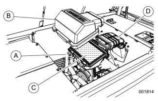
Figure 4-5. Servicing Air Cleaner (13–22 kW)
