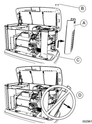
Figure 3-3. Intake Side Panel Removal
