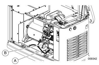
Figure 4-2. Oil Filter and Drain Location (13–16 kW)
