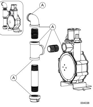
Figure 4-11. Connection Points to Leak Check
