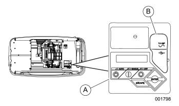
Figure 3-8. Generator Control Panel
