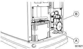
Figure 4-10. Cleaning the Sediment Trap
