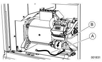
Figure 4-1. Oil Filter and Drain Location (10 kW)
