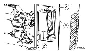
Figure 4-4. Servicing Air Cleaner (10 kW)
