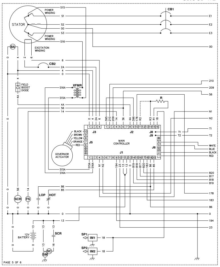
REVISION: A DATE: 09/20/19 SCHEMATIC - DIAGRAM AC HSB EVO2 50HZ 3PH AU DRAWING #: A0000385327
