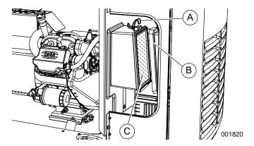
Figure 4-4. Servicing Air Cleaner (10 kW)
