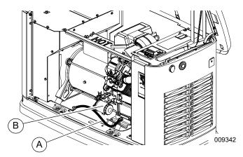
Figure 4-2. Oil Filter and Drain Location (13-16 kW)
