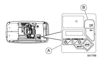
Figure 3-8. Generator Control Panel
