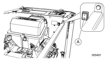
Figure 3-7. Internal Auxiliary Shutdown Switch (13–22kW)
