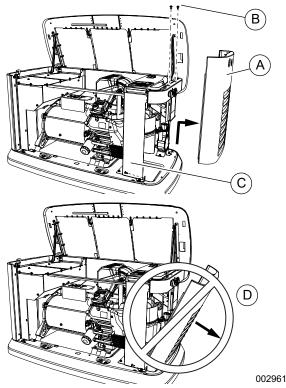
Figure 3-3. Intake Side Panel Removal
