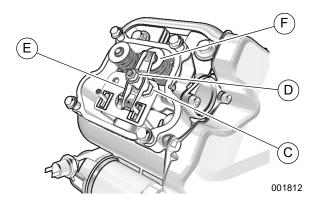
Figure 4-7. Valve Clearance Adjustment (10 kW)
