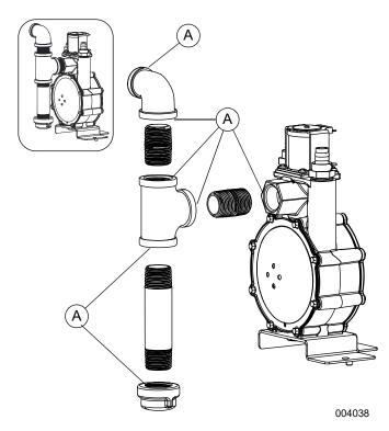
Figure 4-11. Connection Points to Leak Check
