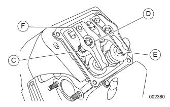
Figure 4-8. Valve Clearance Adjustment (20–22 kW)
