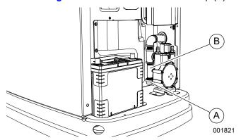
Figure 4-10. Cleaning the Sediment Trap
