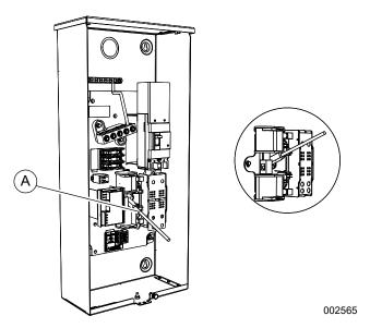
Figure 3-11. Typical Manual Transfer Switch
