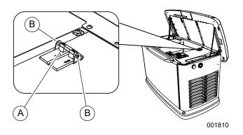
Figure 3-4. Main Line Circuit Breaker (MLCB)
