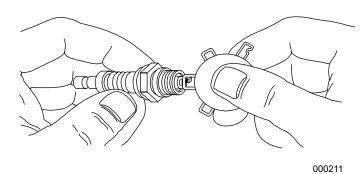
Figure 4-6. Spark Plug Gap Measurement
