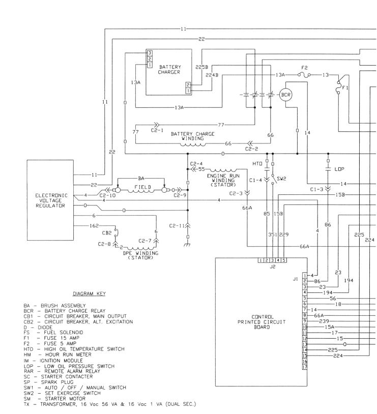
Guardian Air-cooled 7 kW, 12 kW and 15 kW Generators Electrical Schematic - 7 kW - Drawing No. 0D5701-A
