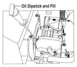
Figure 4.3 — Oil Dipstick and Fill, 12 kW and 15 kW
