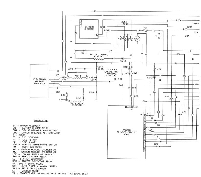
Guardian Air-cooled 7 kW, 12 kW and 15 kW Generators Electrical Schematic - 12kW & 15kW - Drawing No. C7836-B
