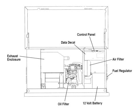
Figure 1.3 - 12 kW/15 kW, V-twin GT-760/GT-990 Engine
