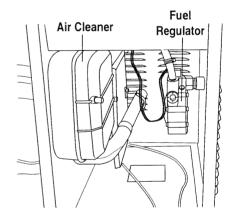
Figure 4.7 — 12 kW and 15 kW Engine Air Cleaner
