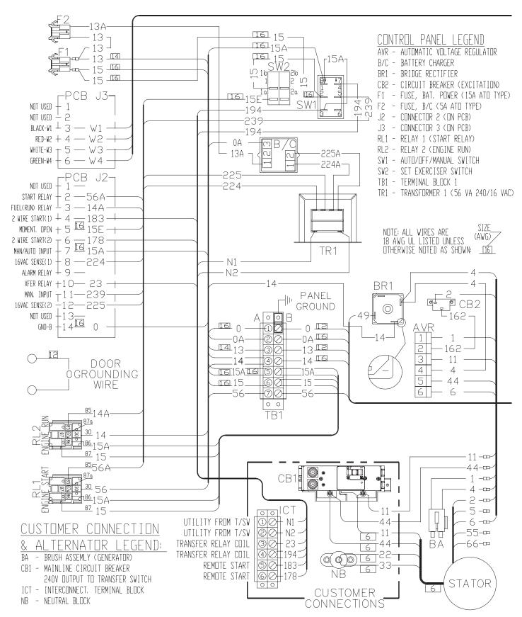
Generac Liquid-cooled 25 kW Generator Wiring Diagram — 2.5L Engine (Model 004990-0) —Drawing No. 0E9982-B
