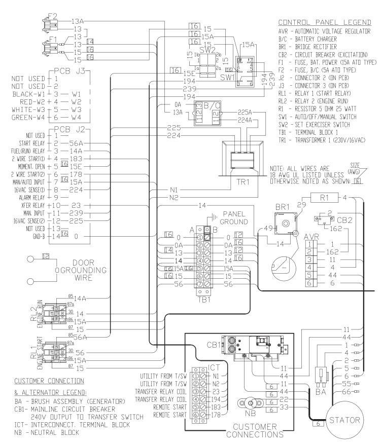
Generac Liquid-cooled 25 kW Generator Wiring Diagram — 2.5L Engine (Model 005078-0) —Drawing No. 0F2452
