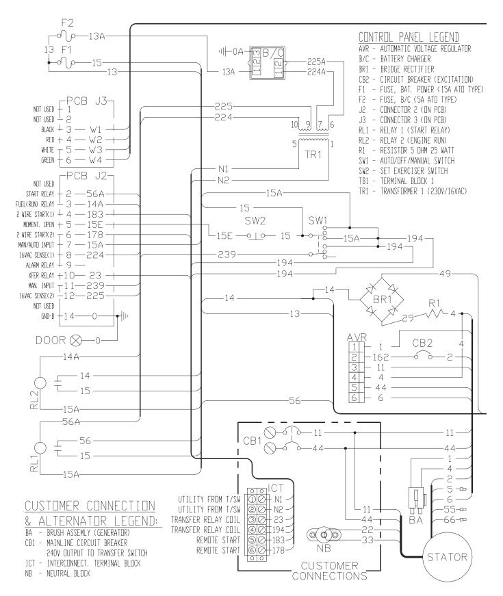
Generac Liquid-cooled 25 kW Generator Electrical Schematic - 2.5L Engine (Models 005048-0 & 005052-0) - Drawing No. 0F1413
