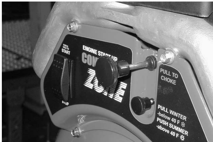
Figure 17 - Full Choke Position
