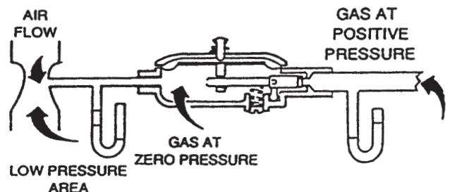
Figure 2.16 – LP Gas Carburetion Diagram
