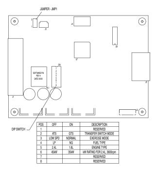
Figure 2 — Dip Switch & Jumper Settings (New Revision)
