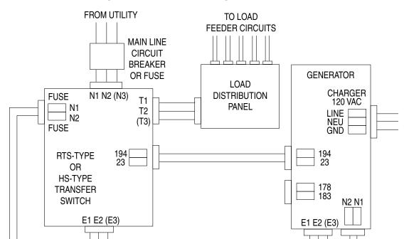
Figure 4 - Connection Diagram (ATS Mode)
