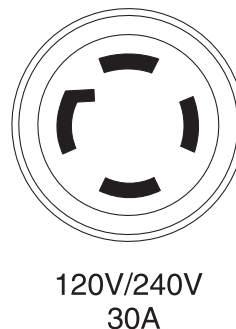
Figure 8 - 120/240 VAC, 30 Amp Receptacle
