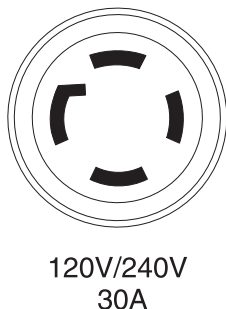
Figure 7 - 120/240 VAC, 30 Amp Receptacle
