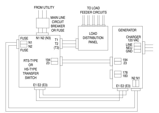
Figure 3 - Connection Diagram (ATS Mode)
