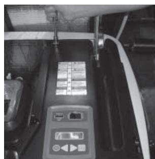
3. Remove the two screws securing the connection area cover, and remove the cover.
