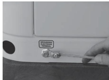
6. Connect an approved ground strap to the grounding lug on the base frame and to an approved earth ground or grounding rod as specified by local regulations.
