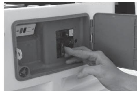
6. Allow the engine to warm up, then switch the generator's main breaker to the ON position. The generator is now supplying electricity to the lower half of the load center but is not carrying any load.
