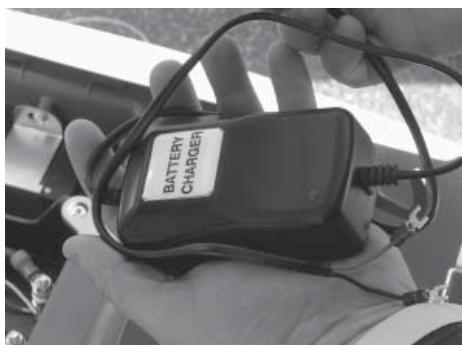
1. The generator battery charger is to be installed in the generator when using a GenReady load center. Refer to the Battery Charger Installation Guide for details.
