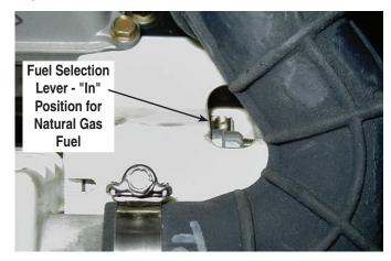
Figure 1.6 - 10kW, GT-530 (Inlet Hose Slid Back)
