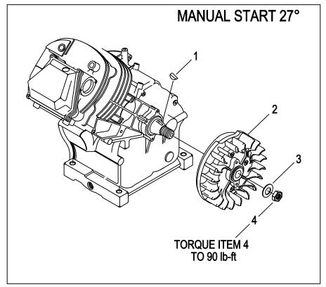
EXPLODED VIEW: FLYWHEEL OPTION, 410cc MANUAL START DRAWING #: 0C4000A
