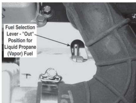
4. Slide the fuel selector pin on the carburetor out towards the back of the enclosure.
