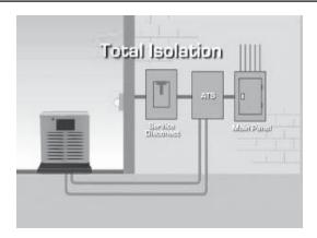
1. The generator will be backing up all electrical loads within the panel, so the amperage rating of the transfer switch must be equal to or greater than the amperage rating of the normal utility service.
