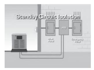
1. The generator powers only designated circuits that are grouped together and wired into a separate priority distribution panel. The transfer switch is installed between the main distribution panel and the priority panel.
