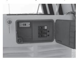
4. The circuit breaker is attached to the exterior access panel.
