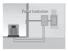
2. A service rated transfer switch is installed between the service and the main distribution panel. The service rated switch becomes the main service so no service disconnect is needed. The existing main distribution panel becomes a subpanel.
