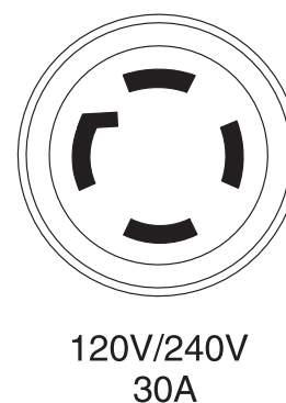
Figure 7 - 120/240 VAC, 30 Amp Receptacle
