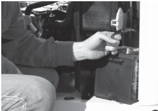
1. Before purchasing a battery for the generator, refer to the generator Owner's Manual for a list of recommended batteries. Follow all of the procedures and safety precautions in the Owner's Manual when installing the battery.
