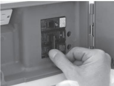
3. Switch the generator's main circuit breaker OFF and put the mode switch in the OFF position.
