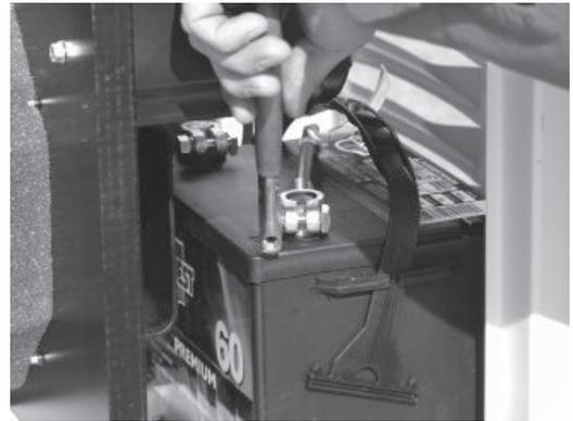
1. The generator was configured for natural gas operation at the factory. Switching over to LP Vapor is a simple procedure. On units with the 8 KVA unit engine, begin by disconnecting and removing the battery if installed. Follow all of the procedures and safety precautions in the generator Owner's Manual when installing and connecting, or disconnecting the battery.
