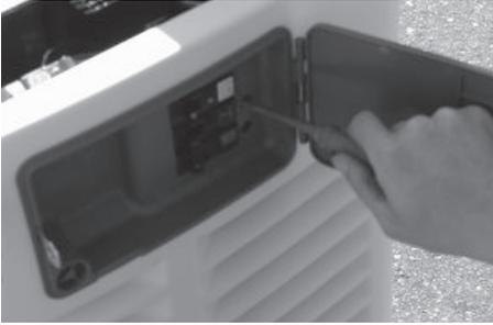
4. The circuit breaker is attached to the exterior access panel.
