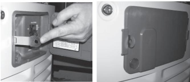
5. Locate the metal hasp that is packaged in the owner's manual bag. Insert the hasp in the slot located on the left side of the external circuit breaker box. Be sure that the clip of the hasp is facing toward the front of the generator. If desired, lock the external box.
