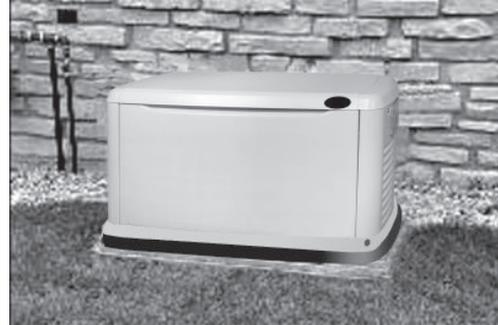
1. Locate the mounting area as close as possible to the transfer switch and fuel supply. Leave adequate room around the area for service access (check local code), and place high enough to keep rising water from reaching the generator. Choose an open space that will provide adequate and unobstructed airflow (see the "Location" section in the Owner's Manual).
