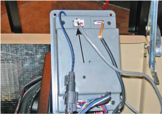
Figure 5B — Plug Wire Harness into 8-pin Header
