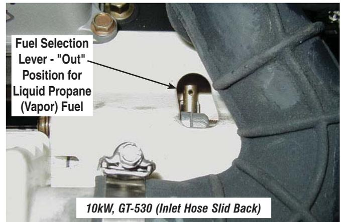
2. For 10kW units: Loosen clamp and slide back the air inlet hose.
