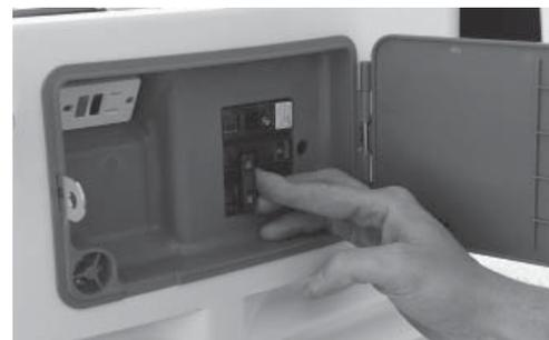
12. Switch the generator's main breaker to the ON position and put the mode switch in AUTO.
