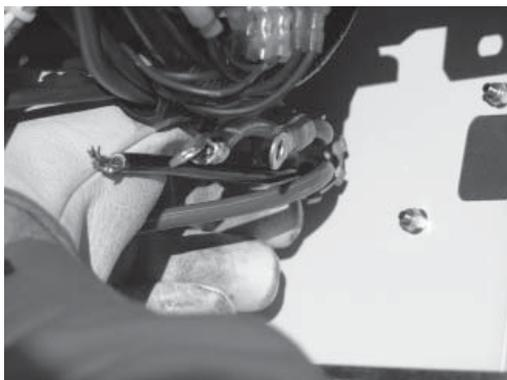
2. Feed the wires through the back of the generator and secure the conduit with the lock nut.
