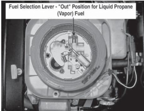
6. On all other models, simply remove the air cleaner cover and slide the fuel selector pin outward from the natural gas to the LP position.
