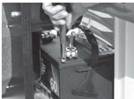
1. The generator was configured for natural gas operation at the factory. Switching over to LP Vapor is a simple procedure. On models with a single cylinder engine, begin by disconnecting and removing the battery if installed. Follow all of the procedures and safety precautions in the generator Owner's Manual when removing and/or installing the battery.
