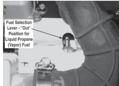
4. Slide the fuel selector pin on the carburetor out towards the back of the enclosure.
