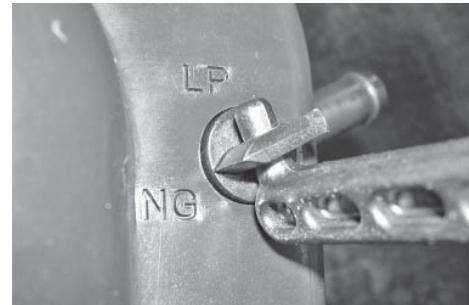
2. Take the plastic T-handle fuel selector in the poly bag supplied with the generator and locate the selector tab on the air box cover. Insert the pin end into the hole in the selector tab and pull outward to overcome spring pressure. Then twist clockwise 90 degrees and allow the selector to return in once aligned with the LP position.
