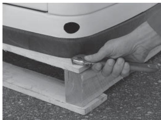
3. Inspect the generator for shipping damage and if necessary, file a claim with the shipper.
