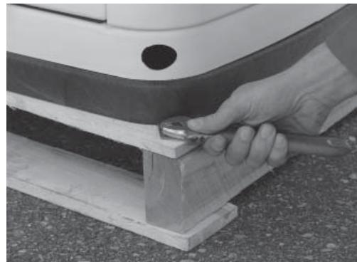
3. Inspect the generator for shipping damage and if necessary, file a claim with the shipper. Remove the bands holding the generator to the wooden pallet.
