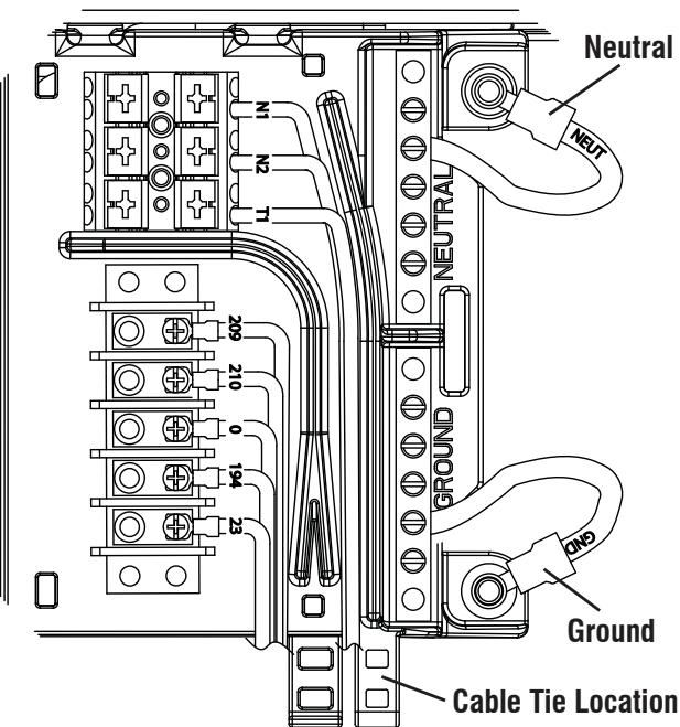
8. Connect the white neutral wire to the neutral bus bar and torque to 35 inch lbs. The torque values are:
