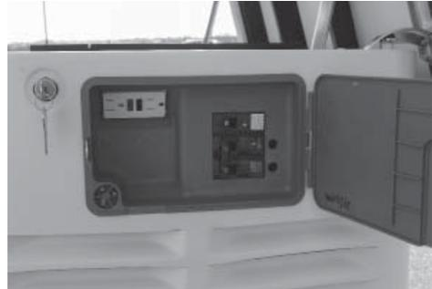
6. The circuit breaker is attached to the exterior access panel.
