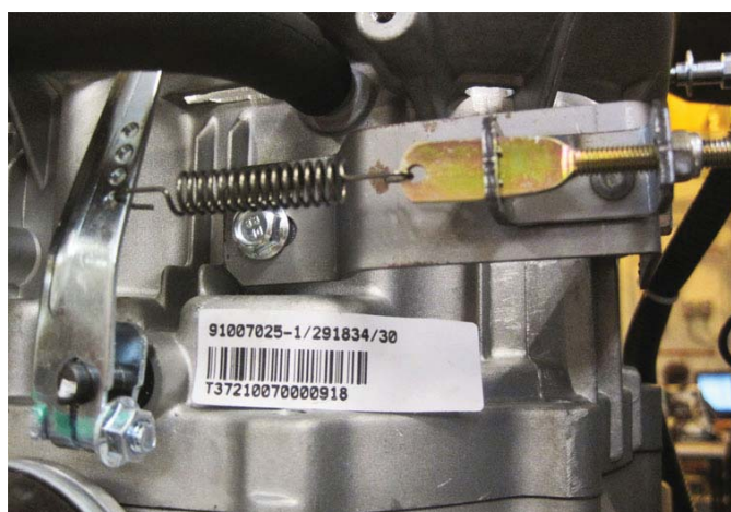
Figure 2.1 — Engine Governor Adjustment Single Cylinder Engines
