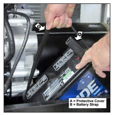
Figure 5-12. Install Battery (2.3L Models)
