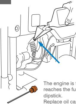
The engine is full when the oil reaches the full mark on the dipstick.
