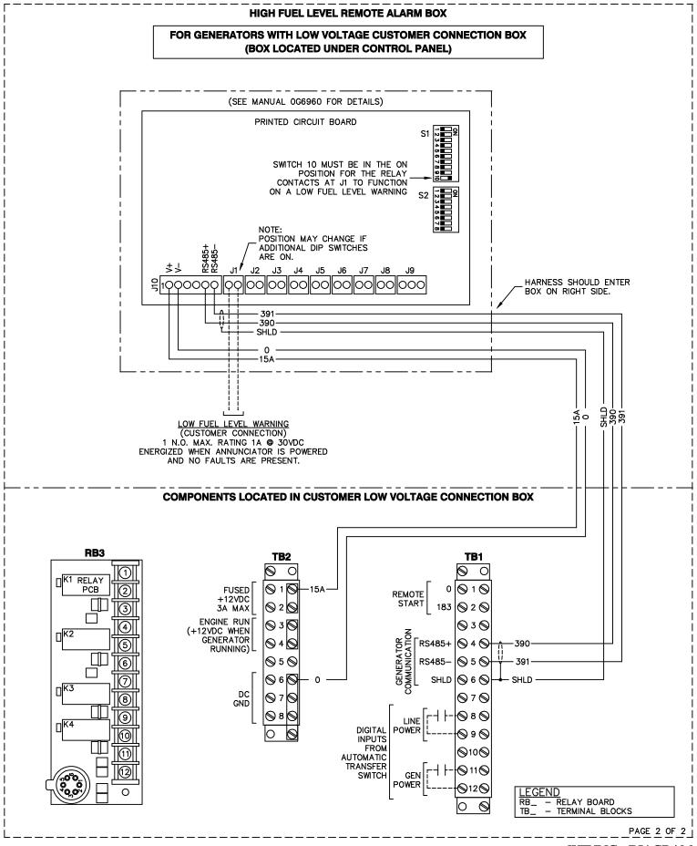
WIRING - DIAGRAM ANNUNCIATOR TO GENSET DRAWING #: 0J2331
