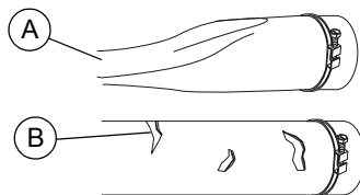
Figure 4-11. Common Suction Hose Faults
