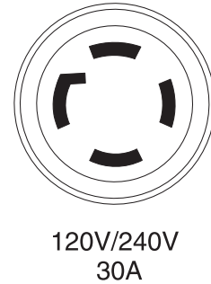
Figure 7 - 120/240 VAC, 30 Amp Receptacle
