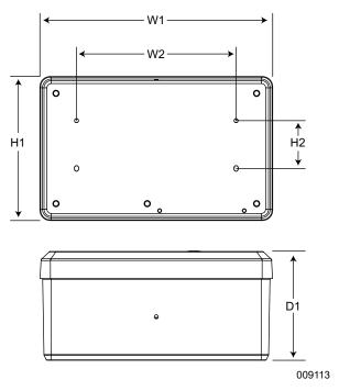
Figure 3-1. Mounting Dimensions
