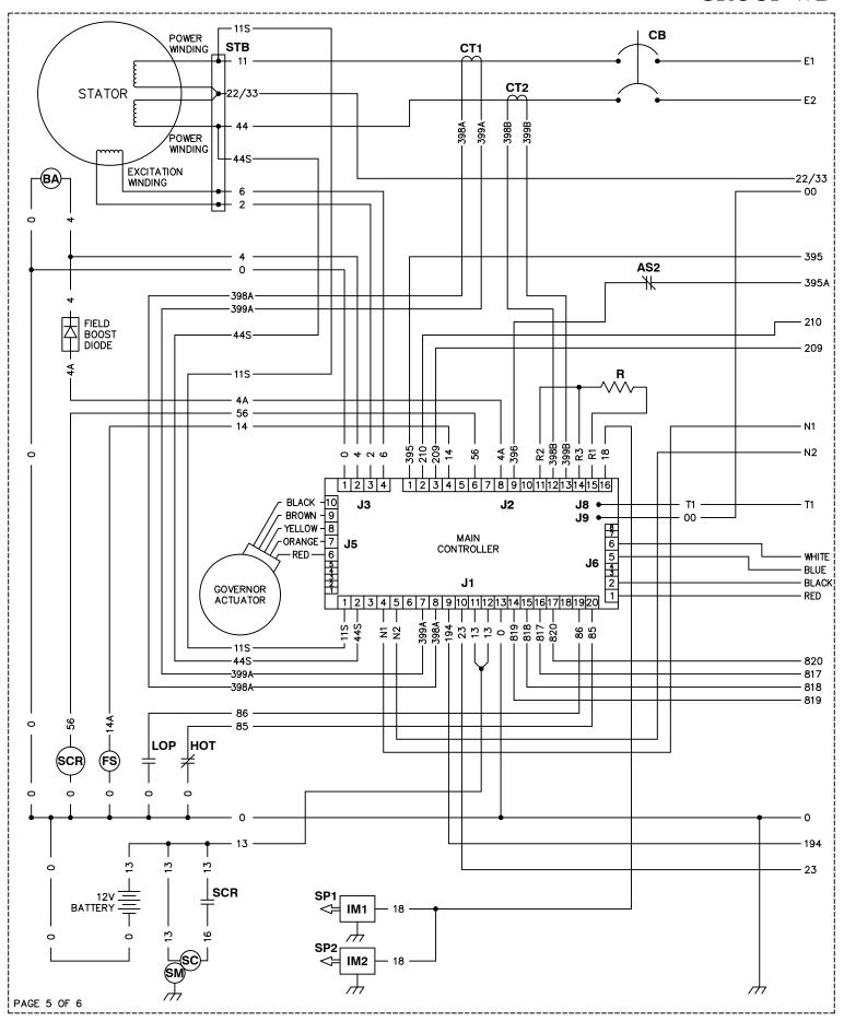
REVISION: A DATE: 10/17/19 SCHEMATIC - DIAGRAM AC HSB EVO2 60HZ 1PH W/ STB DRAWING #: A0000189156
