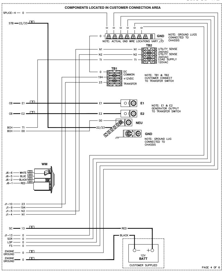
REVISION: A DATE: 10/17/19 WIRING - DIAGRAM AC HSB EVO2 60HZ 1PH W/ STB DRAWING #: A0000189156
