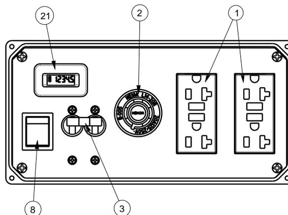
**Figure 4 - Generator Controls**
