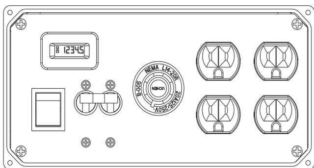
**IMPORTANT:** Do not overload the generator. Also, do not overload individual panel receptacles. These outlets are protected against overload with circuit breakers. If amperage rating of any circuit breaker is exceeded, that breaker opens and electrical output to that receptacle is lost. Read "Don't Overload the Generator" carefully.
