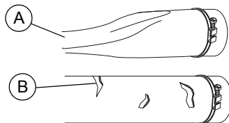
Figure 4-11. Common Suction Hose Faults
