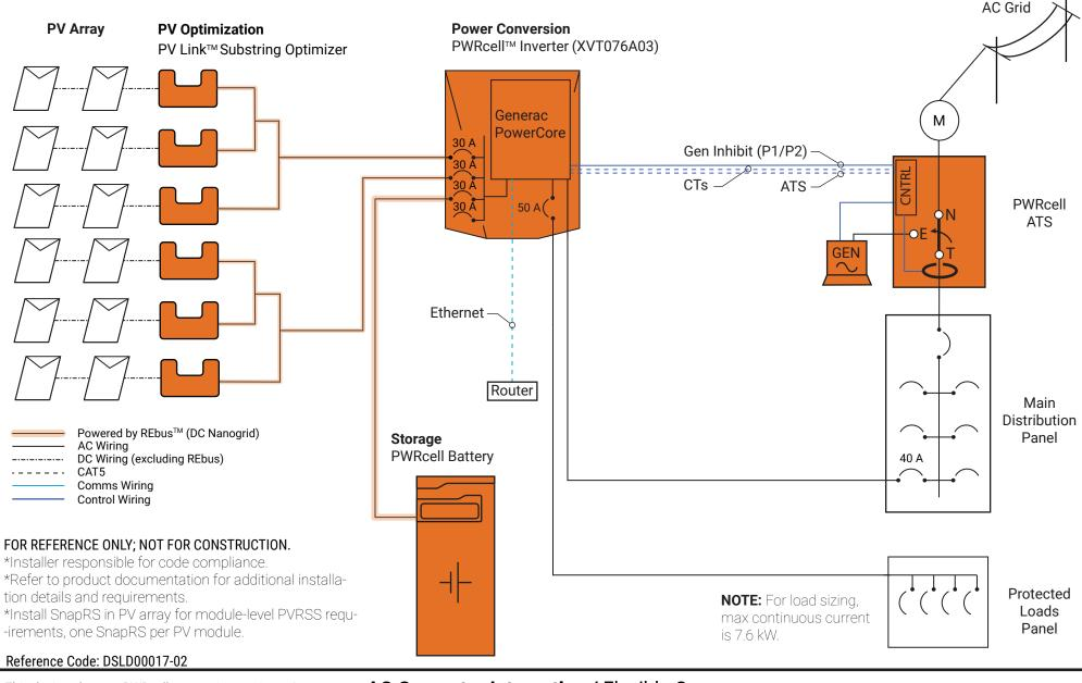
This design shows a PWRcell system integrating a Generac generator. The inverter backs up a protected loads panel when the generator is not turned on. When turned on, the generator supports all house loads and can charge the PWRcell Battery. It is suitable for most residential 120V/240 V services. Recommended generator control modes: "Single Transfer" or "Source Cycling".
