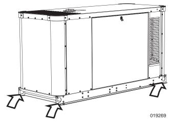
Figure 2-1. Lifting Points (Four Places)
